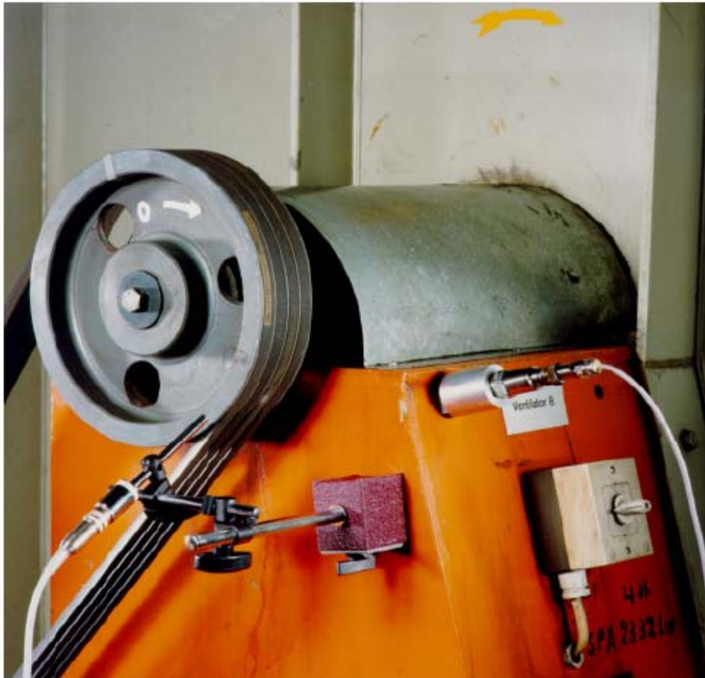
Figure 3.9: The reference mark attached to the pulley and the photo-electric sensor mounted in the magnetic stand (left) in the example. The acceleration sensor was mounted by magnet on the bearing support structure.
